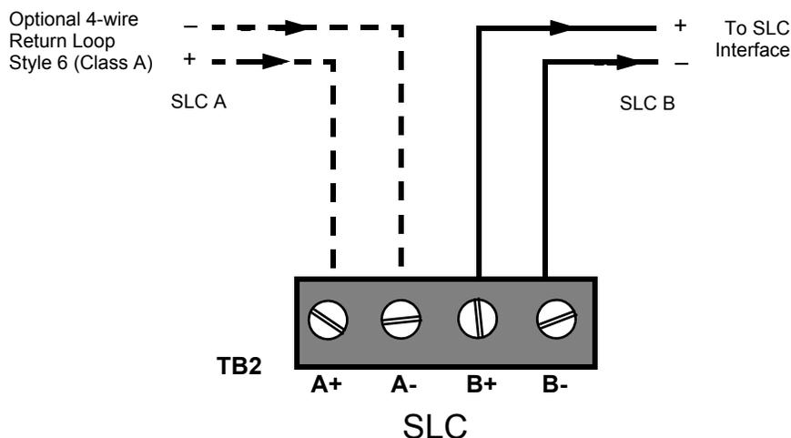
Figure 2.14 Connecting to the SLC Interface TB2
