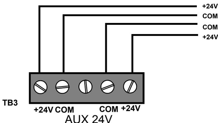
Figure 2.13 Connecting to the AUX 24V Output TB3
